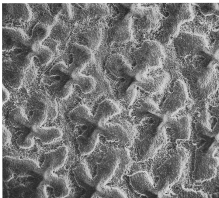
Figure 1 A scanning electron microscope image showing the dendrite structure on a complex Ni-Ta-Cr-Mn system (approximate composition Ni 57, Ta 21, Cr 15 and Mn 7 wt %) unidirectionally solidified in the following condition: thermal gradient 80^{\circ}\text{C cm}^{-1} , solidification rate 9.5\text{ cm h}^{-1} . The image is of a transversal section of an ingot ( \phi , 12 mm) strongly attacked by electrolytic etching ( \times 100 ).
